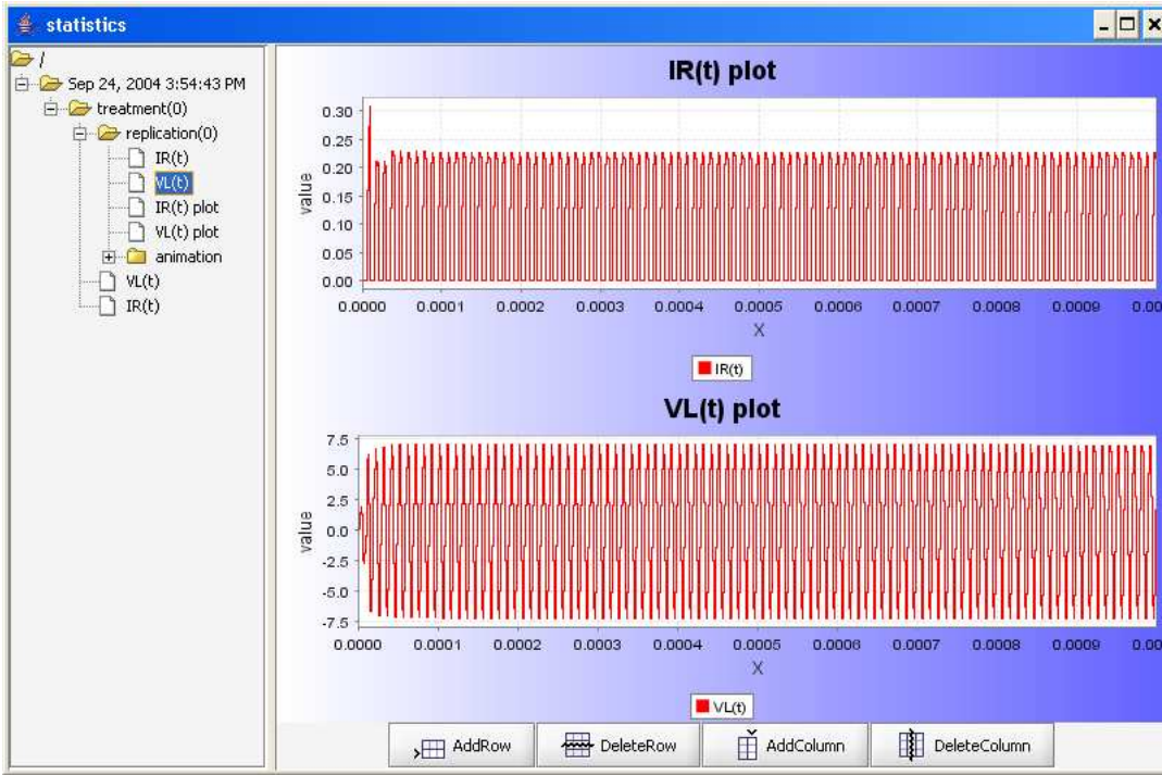
Fig. 6.14: Results of simulating the stiff system over t=[0, 10^{-4}] sec.
